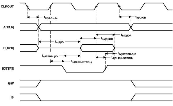
Figure 7. Parallel I/O Port Read (IOSTRB = 0)
