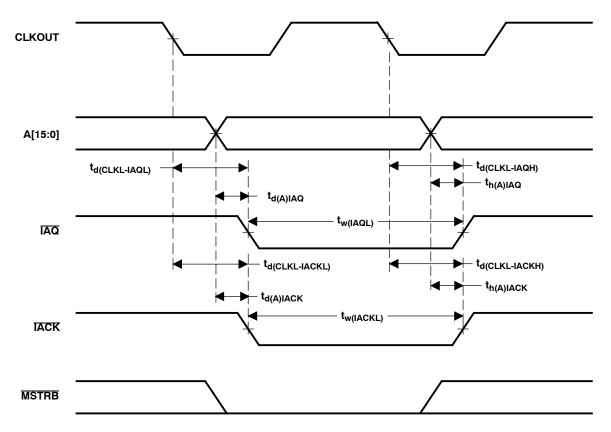
Figure 18. Instruction Acquisition (IAQ) and Interrupt Acknowledge (IACK) Timing
