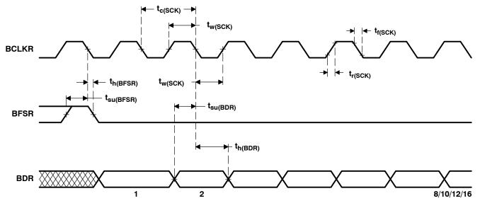
Figure 24. Buffered Serial Port Receive Timing
