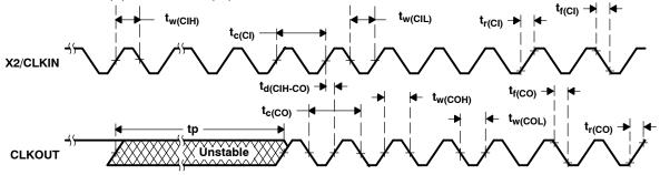
Figure 4. External Multiply-by-One Clock Timing
