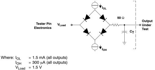
$C_{T}$ = 40 pF typical load circuit capacitance.
