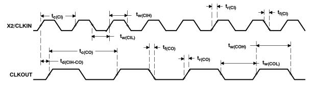
Figure 3. External Divide-by-Two Clock Timing
