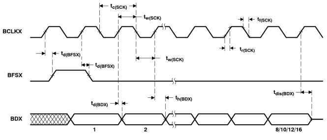
Figure 26. Buffered Serial Port Transmit Timing of Internal Clocks and Internal Frames
