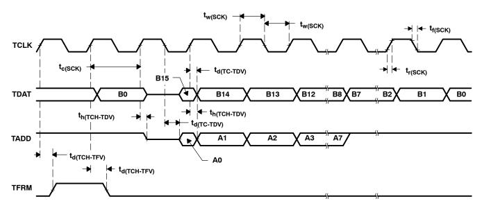
Figure 28. Serial-Port Transmit Timing in TDM Mode
