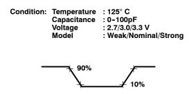
Figure 9. Rise and Fall Time Diagram
