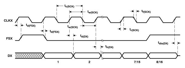
Figure 23. Serial Port Transmit Timing With Internal Clocks and Frames
