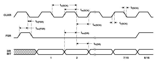
Figure 21. Serial Port Receive Timing
