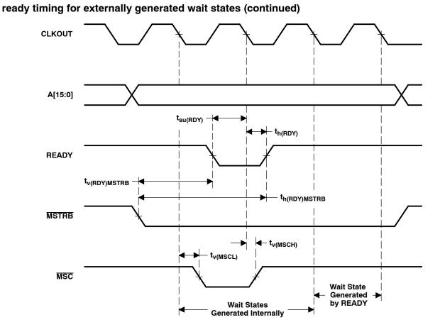
Figure 10. Memory Read With Externally Generated Wait States
