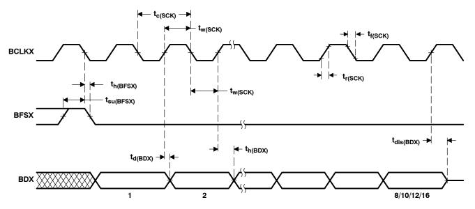
Figure 25. Buffered Serial Port Transmit Timing of External Clocks and External Frames
