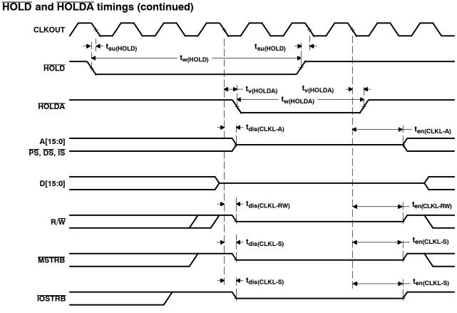
Figure 14. HOLD and HOLDA Timing (HM = 1)
