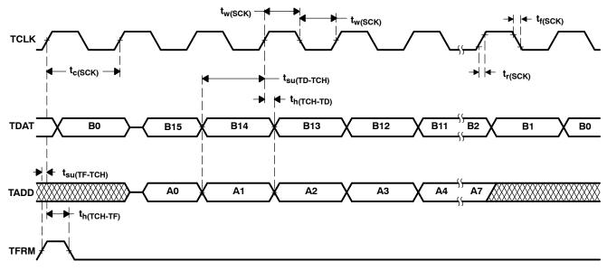
serial-port receive timing in TDM mode (continued)
