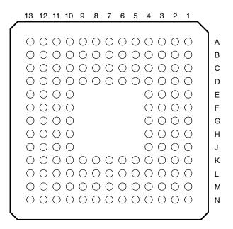
The pin assignments table to follow lists each signal quadrant and BGA ball pin number for the 144-pin BGA package.
