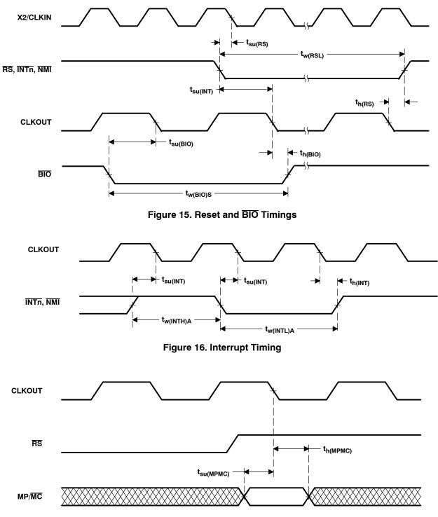
Figure 17. MP/MC Timing
