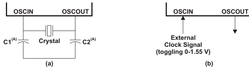
Figure 5-3. Recommended Crystal/Clock Connection
