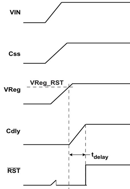
**Figure 13. Power-On Condition and Reset Line**
