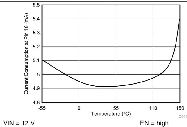
**Figure 9. Current Consumption With Temperature**
