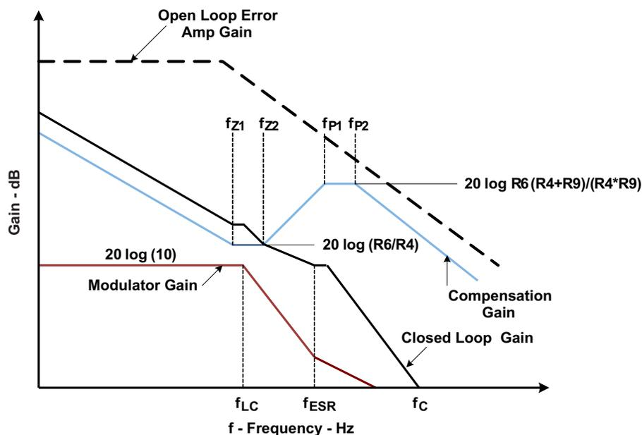
**Figure 16. Bode Plot of Converter Gain Plot**
