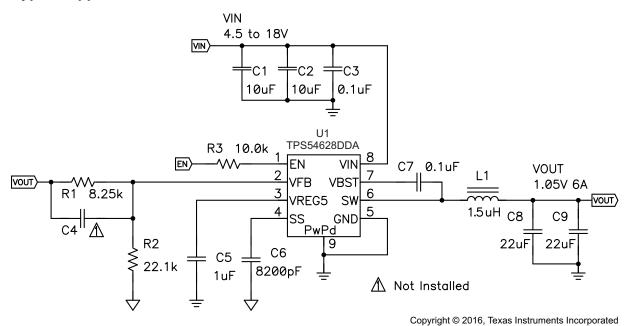
Figure 12. Simplified Application Schematic Example
