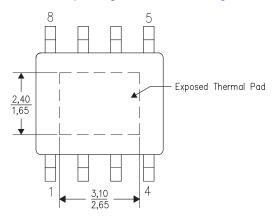
Figure 19. Thermal Pad Dimensions
