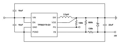
Figure 30. -5-V Inverting Power Supply
