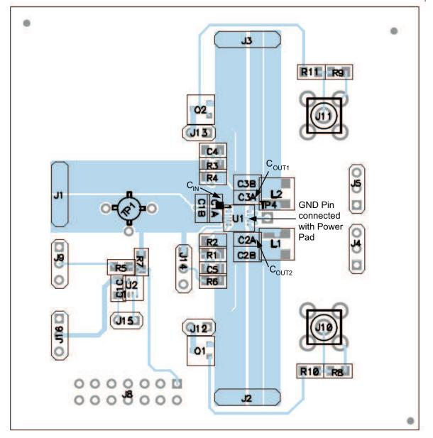
Figure 49. PCB Layout
