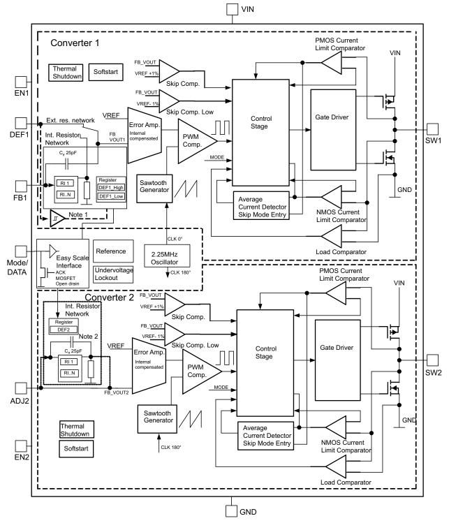
(1) In fixed output voltage version, the PIN DEF\_1 is connected to an internal digital input and disconnected from the error amplifier
