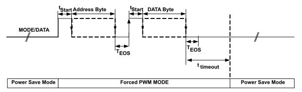
Figure 13. MODE/DATA Pin: Power Save Mode/Interface Communication
