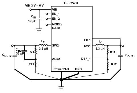
Figure 48. Layout Diagram
