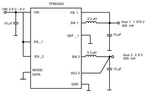
Figure 45. TPS62403 1.575V/2.8V Outputs
