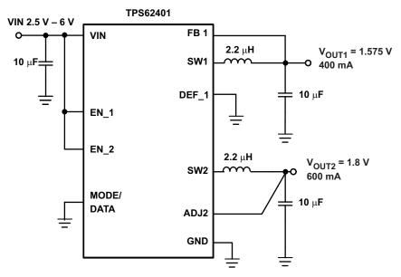
Figure 43. TPS62401 Fixed 1.575V/1.8V Outputs
