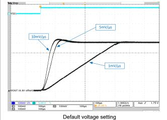
Figure 9-12. DVS by VSEL, Different Ramp Speed Settings
