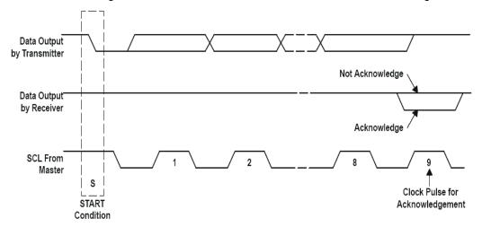
Figure 8-5. Acknowledge on the I<sup>2</sup>C Bus
