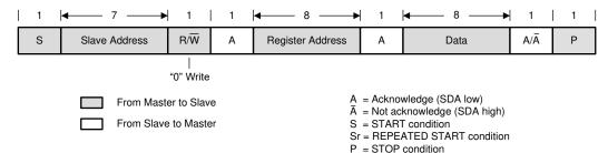
Figure 8-7. "Write" Data Transfer Format in Standard-, Fast, and Fast-Plus Modes
