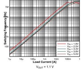
Figure 9-8. Switching Frequency
