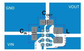
Figure 9-20. PCB Layout Example
