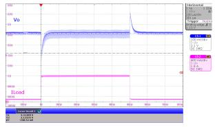
$$V_{I}=3.3~V,~V_{O}=3.3~V \qquad \begin{array}{c} I_{O}~from~100~mA~to\\ 1~A~t_{r}=1~\mu s,~t_{f}=\\ 1~\mu s \end{array} \qquad \begin{array}{c} MODE=High\\ \end{array}$$
