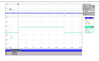
$$\label{eq:v1} I_O = 0.5 \; A \qquad \qquad \begin{array}{l} V_I \; \text{from 3 V to 3.6} \\ V \; t_r = 1 \; \mu \text{s, } t_f = 1 \\ \mu \text{s} \end{array} \quad \text{MODE} = \text{High}$$
