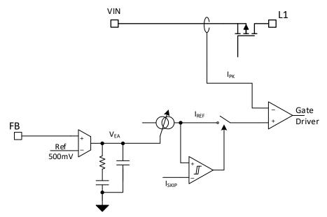
Figure 9-1. Control Loop Architecture Scheme
