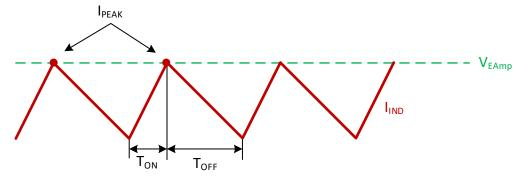
Figure 9-7. Peak-Current Boost Operation
