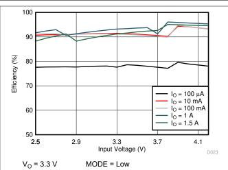
Figure 10-8. Efficiency versus Input Voltage (PWM Only)
