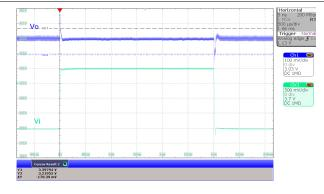
V<sub>I</sub> from 2.2 V to  $I_0 = 1 A$  $4.2 \text{ V t}_r = 1 \text{ } \mu\text{s}, \text{ } t_f$ MODE = High = 1 µs
