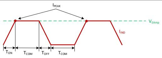
Figure 9-8. Peak-Current Buck-Boost Operation
