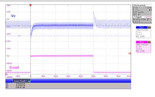
$$V_{I} = 2.5 \text{ V, } V_{O} = 3.3 \qquad \begin{array}{l} I_{O} \text{ from 100 mA to} \\ 1 \text{ A } t_{r} = 1 \text{ } \mu \text{s, } t_{f} = 1 \\ \mu \text{s} \end{array} \qquad \text{MODE} = \text{Low}$$
