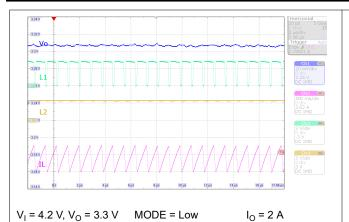
Figure 10-20. Switching Waveforms, PWM Buck Operation
