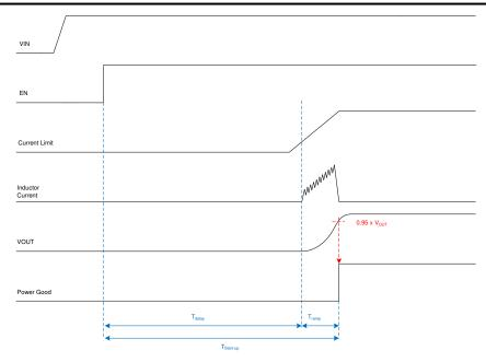
Figure 9-4. Device Start-up Scheme
