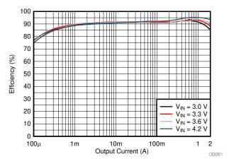
Efficiency vs Output Current ( $V_0 = 3.3 \text{ V}$ )
