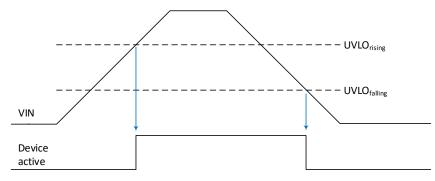
Figure 9-3. Rising and Falling Undervoltage Lockout Behavior
