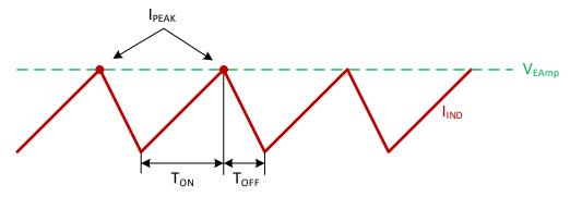
Figure 9-9. Peak-Current Buck Operation
