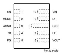
Figure 7-1. 10-Pin DLA Package (Top View)
