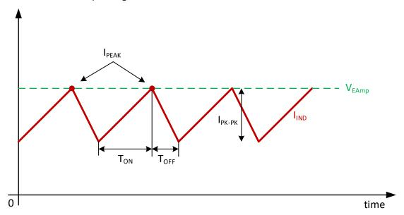
Figure 9-5. Peak-Current Architecture Operation
