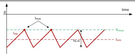
Figure 9-6. Peak-Current Operation, Reverse Current
