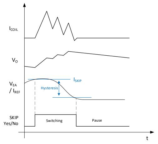
Figure 9-10. Power Safe Mode Operation Curves
