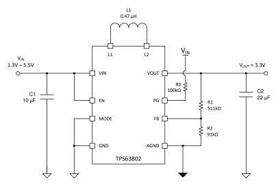
Figure 10-1. 3.3 V<sub>OUT</sub> Typical Application
