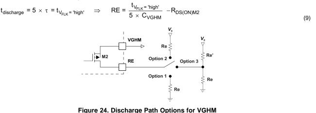
Options 2 and 3 from Figure 24 work like option 1 explained above. When M2 is turned on,  $V_{GHM}$  discharges with a slope set by Re from  $V_{GH}$  level down to  $V_S$  in option 2 configuration and in option 3 configuration down to the voltage set by the resistor divider. The discharging slope is set by Re resistor(s).
