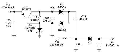
Figure 22. Partially Regulated External Negative
