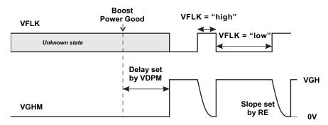
Figure 23. Gate Voltage Shaping Timing
