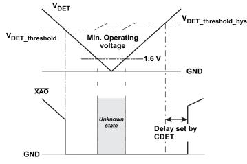
Figure 25. Voltage Detection and XAO Pin
