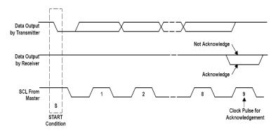
Figure 33. Acknowledge on the I<sup>2</sup>C Bus
