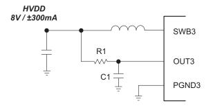
Figure 29. Connection of the snubber circuit for Buck 3
