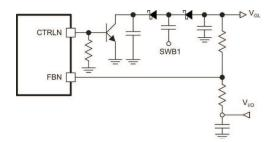
Figure 26. Negative Charge Pump Application Circuit
