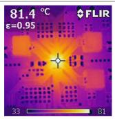
VIN = 12 V, VOUT1 = 1.5 V/3 A, VOUT2 = 1.2 V/2 A, VOUT3 = 2.5 V/2 A.
