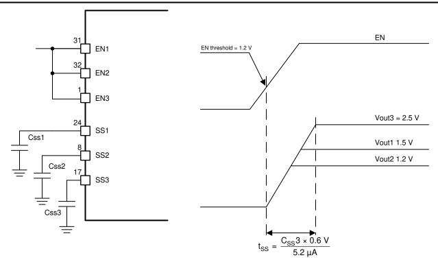
Figure 7-7. Simultaneous Start-up Sequence Using SSx Pins
