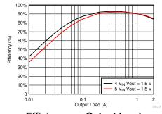
**Efficiency vs Output Load**
