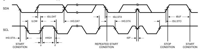
Figure 7-14. I<sup>2</sup>C Interface Timing Diagram
