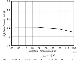
Figure 6-19. Buck2 High-Side Current Limit vs Temperature
