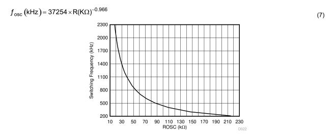
Figure 7-12. ROSC vs Switching Frequency
