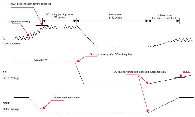
Figure 7-11. Overcurrent Protection
