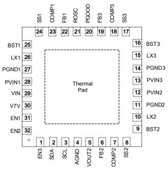
There is no electric signal down bonded to thermal pad inside IC. Exposed thermal pad must be soldered to PCB for optimal thermal performance.
