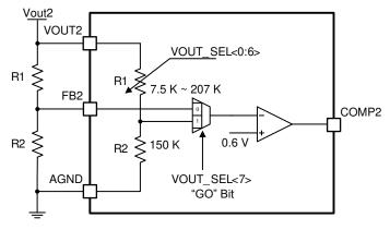
Figure 7-2. Voltage Divider Circuit
