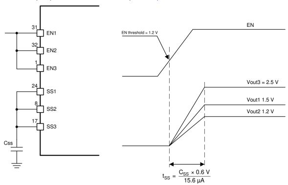
Figure 7-6. Ratiometric Power-Up Using SSx Pins
