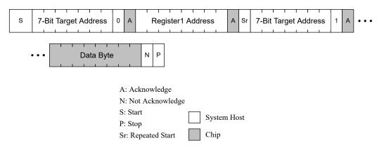
Figure 7-16. I<sup>2</sup>C Read Data Format
