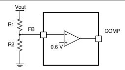
Figure 7-1. Voltage Divider Circuit
