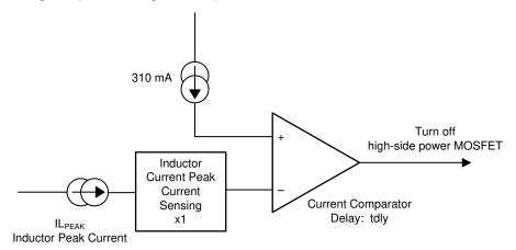
Figure 7-10. PSM Current Comparator
