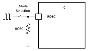
Figure 7-13. Works With Resistor Mode and Synchronization Mode
