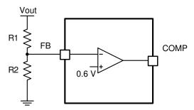
Figure 8-1. Voltage Divider Circuit
