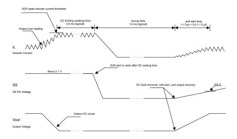
Figure 8-11. Overcurrent Protection
