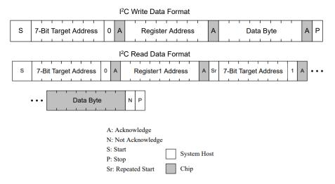
Figure 8-13. I<sup>2</sup>C Write and Read Data Format
