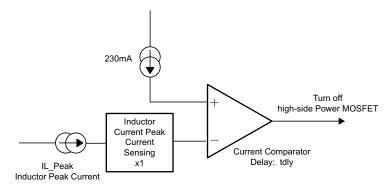
Figure 8-10. PSM Current Comparator
