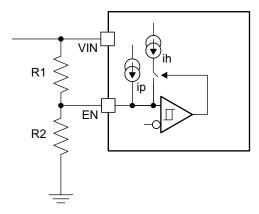
Figure 8-3. Adjustable VIN UVLO
