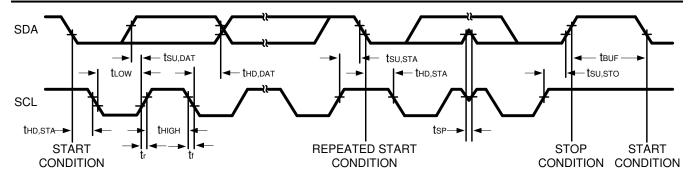
Figure 8-12. I<sup>2</sup>C Interface Timing Diagram
