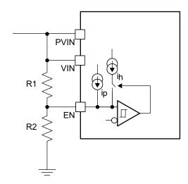
Figure 8-5. Adjustable VIN and PVIN UVLO
