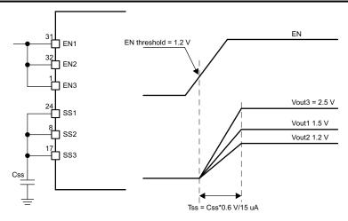
Figure 8-6. Ratiometric Power-Up Using SSx Pins
