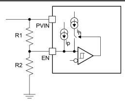
Figure 8-4. Adjustable PVIN UVLO, VIN > 4.5 V
