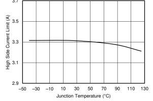
Figure 7-19. Buck2 High-Side Current Limit vs Temperature
