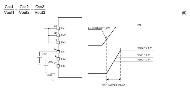
Figure 8-7. Simultaneous Startup Sequence Using SSx Pins
