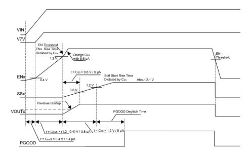
Figure 8-8. Startup Power Sequence
