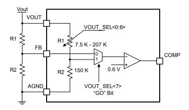
Figure 8-2. Voltage Divider Circuit
