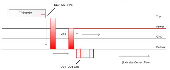
Figure 24. DEV\_OUT Recommended Routing
