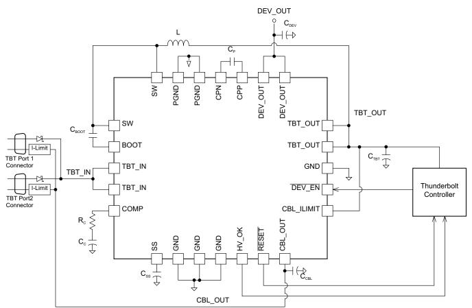
Figure 22. Typical Application (Dual-Port Bus-Powered Thunderbolt™ Device)
