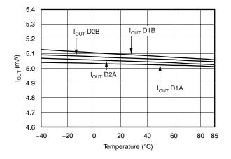
R<sub>SET</sub> = open Figure 14. TPS75105 Output Current vs Temperature
