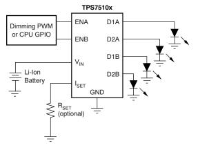
Figure 13. Typical Application Diagram
