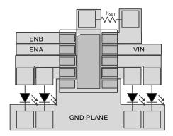
Figure 15. Layout Example for the WSON (DSK) Package
