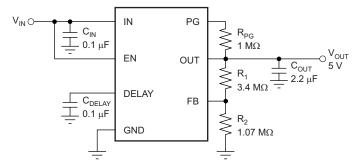
Figure 15. Adjustable Operation
