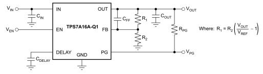
Figure 14. The TPS7A16A-Q1 Circuit as an Adjustable Regulator Schematic
