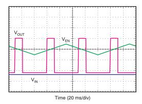
Figure 18. Enable Pin Positive and Negative Threshold
