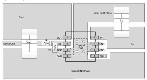
NOTE:  $C_{IN}$  and  $C_{OUT}$  are size 1208 capacitors, while  $R_1$  and  $R_2$  are size 0402.
