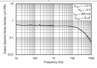
Figure 17. Output Spectral Noise Density
