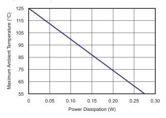
Figure 25. Maximum Ambient Temperature (°C) vs Power Dissipation
