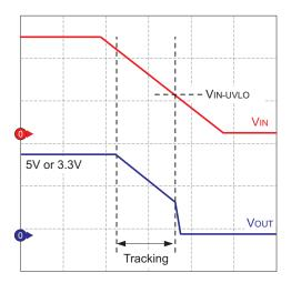
Figure 18. Low Voltage Tracking Operation
