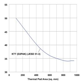
Figure 24.  $R_{\theta JA}$  vs Thermal Pad Area
