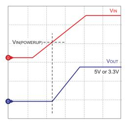
Figure 15. Power-Up Operation
