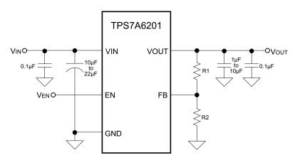
Figure 20. Typical Application Schematic for TPS7A6201-Q1
