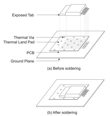
Figure 23. Using Multilayer PCB and Thermal Vias for Adequate Heat Dissipation
