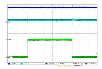
Figure 21. Load Transient Waveform
