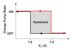
Figure 16. Charge Pump Operation at Light Loads
