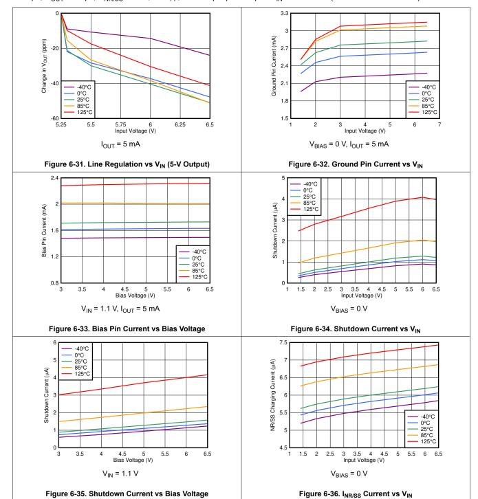
at  $T_A$  = 25°C,  $V_{IN}$  = 1.4 V or  $V_{IN}$  =  $V_{OUT(nom)}$  + 0.4 V (w hichever is greater),  $V_{BIAS}$  = open,  $V_{OUT(nom)}$  = 0.8 V,  $V_{EN}$  = 1.1 V,  $C_{IN}$  = 10  $\mu$ F,  $C_{OUT}$  = 47  $\mu$ F,  $C_{NR/SS}$  = 0 nF, no  $C_{FF}$ , and PG pin pulled up to  $V_{IN}$  with 100  $k\Omega$  (unless otherwise noted)
