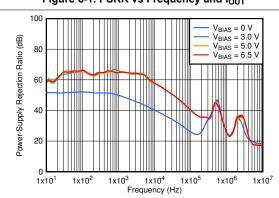
$V_{IN}$  = 1.4 V,  $I_{OUT}$  = 1 A,  $C_{OUT}$  = 47  $\mu$ F || 10  $\mu$ F || 10  $\mu$ F,  $C_{NR/SS}$  = 10 nF,  $C_{FF}$  = 10 nF
