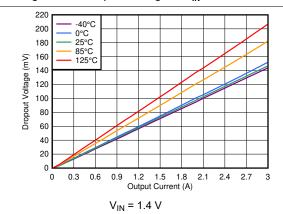
Figure 6-22. Dropout Voltage vs I<sub>OUT</sub> Without Bias
