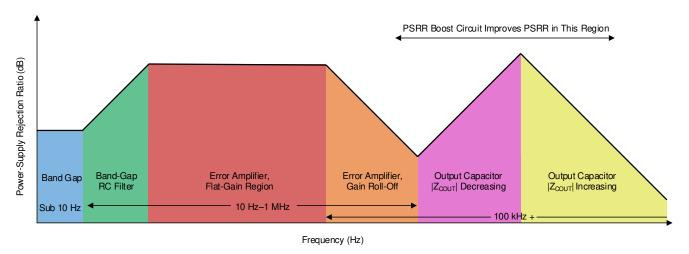
Figure 8-6. Power-Supply Rejection Ratio Diagram
