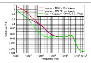
$I_{OUT}$  = 3 A,  $C_{OUT}$  = 47  $\mu$ F || 10  $\mu$ F || 10  $\mu$ F,  $C_{FF}$  = 10 nF, RMS noise BW = 10 Hz to 100 kHz
