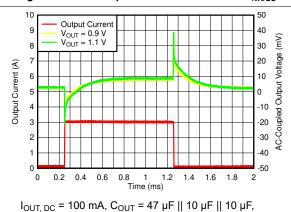
Figure 6-17. Load Transient vs Time and V<sub>OUT</sub> Without Bias
