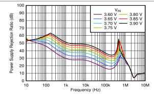
$I_{OUT}$  = 3 A,  $C_{OUT}$  = 47  $\mu$ F || 10  $\mu$ F || 10  $\mu$ F,  $C_{NR/SS}$  = 10 nF, C<sub>FF</sub> = 10 nF
