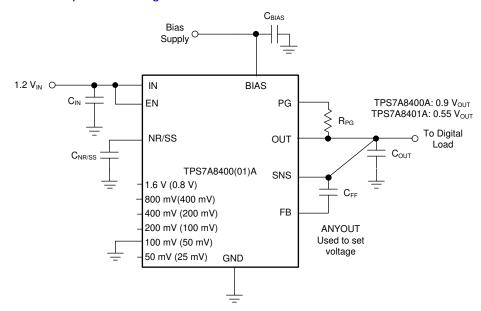
Figure 8-21. TPS7A84A Typical Application
