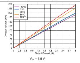
Figure 6-24. Dropout Voltage vs I<sub>OUT</sub> (High V<sub>IN</sub>)
