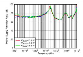
$\begin{aligned} V_{\text{IN}} = V_{\text{OUT}} + 0.3 \ V, \ V_{\text{OUT}} = 1 \ V, \ I_{\text{OUT}} = 3 \ A, \ C_{\text{OUT}} = 47 \ \mu\text{F} \ || \\ 10 \ \mu\text{F} \ || \ 10 \ \mu\text{F}, \ C_{\text{NR/SS}} = 10 \ \text{nF}, \ C_{\text{FF}} = 10 \ \text{nF} \end{aligned}$
