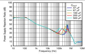
$V_{IN} = 1.4 \text{ V}, V_{BIAS} = 5 \text{ V}, V_{OUT} = 1 \text{ V}, I_{OUT} = 3 \text{ A},$   $C_{NR/SS} = 10 \text{ nF}, C_{FF} = 10 \text{ nF}$
