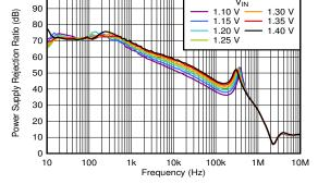
$I_{OUT} = 3 \text{ A}, V_{BIAS} = 5 \text{ V}, C_{OUT} = 47 \mu\text{F} \parallel 10 \mu\text{F} \parallel 10 \mu\text{F},$  $C_{NR/SS} = 10 \text{ nF}, C_{FF} = 10 \text{ nF}$
