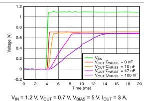
Figure 6-59. Start-Up Waveform vs Time and C<sub>NR/SS</sub>
