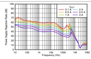
$V_{IN}$  = 5.5 V,  $V_{OUT}$  = 5 V,  $I_{OUT}$  = 3 A,  $C_{OUT}$  = 47  $\mu$ F || 10  $\mu$ F || 10  $\mu$ F,  $C_{NR/SS}$  = 10 nF,  $C_{FF}$  = 10 nF
