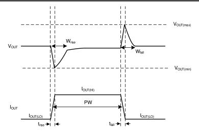
Figure 8-10. Simplified Load Transient Waveform
