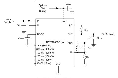
Figure 8-1. Adjustable Operation
