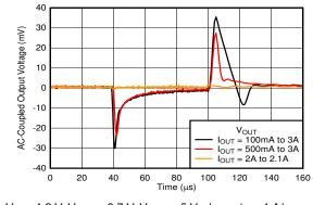
$V_{IN}$  = 1.2 V,  $V_{OUT}$  = 0.7 V,  $V_{BIAS}$  = 5 V, slew rate = 1 A/µs,  $C_{OUT}$  = 47 µF || 10 µF || 10 µF,  $C_{NR/SS}$  =  $C_{FF}$  = 10 nF
