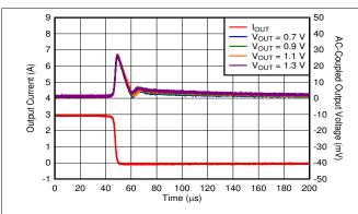
$$\begin{split} V_{\text{IN}} = V_{\text{OUT}} + 0.5 \text{ V}, & V_{\text{BIAS}} = 5 \text{ V}, & I_{\text{OUT}} = 3 \text{ A to } 100 \text{ mA}, \\ \text{slew rate} = 1 \text{ A/\mu s}, & C_{\text{NR/SS}} = C_{\text{FF}} = 10 \text{ nF}, \\ & C_{\text{OUT}} = 47 \text{ } \mu \text{F} \text{ } || & 10 \text{ } \mu \text{F} \text{ } || & 10 \text{ } \mu \text{F} \end{split}$$
