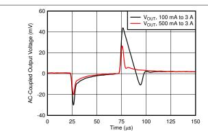
$V_{IN}$  = 1.2 V,  $V_{BIAS}$  = 5 V,  $C_{OUT}$  = 47  $\mu$ F || 10  $\mu$ F || 10  $\mu$ F,  $V_{OUT} = 0.9 \text{ V}$ ,  $C_{NR/SS} = C_{FF} = 10 \text{ nF}$ , slew rate = 1 A/ $\mu$ s
