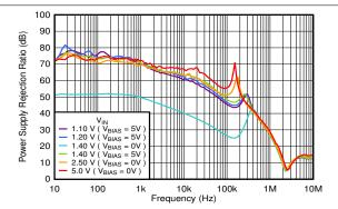
$I_{OUT}$  = 1 A,  $C_{OUT}$  = 47  $\mu$ F || 10  $\mu$ F || 10  $\mu$ F,  $C_{NR/SS}$  = 10 nF, C<sub>FF</sub> = 10 nF
