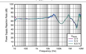
$V_{IN} = V_{OUT} + 0.3 \text{ V}, V_{OUT} = 1 \text{ V}, I_{OUT} = 3 \text{ A}, C_{OUT} = 47 \text{ }\mu\text{F} \text{ }|| 10 \text{ }\mu\text{F}, C_{NR/SS} = 10 \text{ }n\text{F}, C_{FF} = 10 \text{ }n\text{F}$
