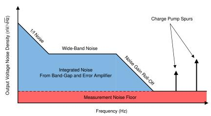
Figure 8-7. Output Voltage Noise Diagram
