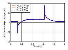
$V_{OUT} = 5 \text{ V, } I_{OUT, DC} = 100 \text{ mA, } I_{OUT} = 100 \text{ mA to } 3 \text{ A, } C_{OUT} = 47 \text{ } \mu\text{F } || 10 \text{ } \mu\text{F, } || 10 \text{ } \mu\text{F, } C_{NR/SS} = C_{FF} = 10 \text{ } n\text{F}$
