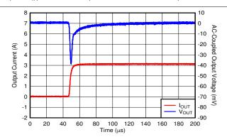
$V_{\text{IN}} = V_{\text{OUT}} + 0.5 \text{ V}, V_{\text{OUT}} = 0.7 \text{ V}, I_{\text{OUT}} = 100 \text{ mA to } 3 \text{ A}, \\ C_{\text{OUT}} = 47 \text{ }\mu\text{F} \text{ }|| 10 \text{ }\mu\text{F} \text{ }|| 10 \text{ }\mu\text{F}, C_{\text{NR/SS}} = C_{\text{FF}} = 10 \text{ nF, slew rate} \\ = 1 \text{ A/}\mu\text{s}$
