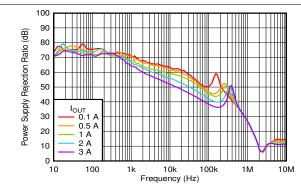
$V_{IN}$  = 1.1 V,  $V_{BIAS}$  = 5 V,  $C_{OUT}$  = 47  $\mu$ F || 10  $\mu$ F || 10  $\mu$ F,  $C_{NR/SS}$  = 10 nF,  $C_{FF}$  = 10 nF
