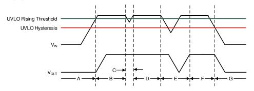
Figure 8-4. Typical UVLO Operation
