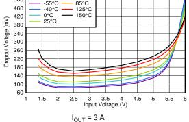
Figure 6-66. Dropout Voltage vs V<sub>IN</sub> Without Bias
