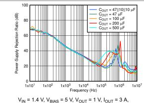
$V_{IN} = 1.4 \text{ V}, V_{BIAS} = 5 \text{ V}, V_{OUT} = 1 \text{ V}, I_{OUT} = 3 \text{ A}$  $C_{NR/SS} = 10 \text{ nF}, C_{FF} = 10 \text{ nF}$
