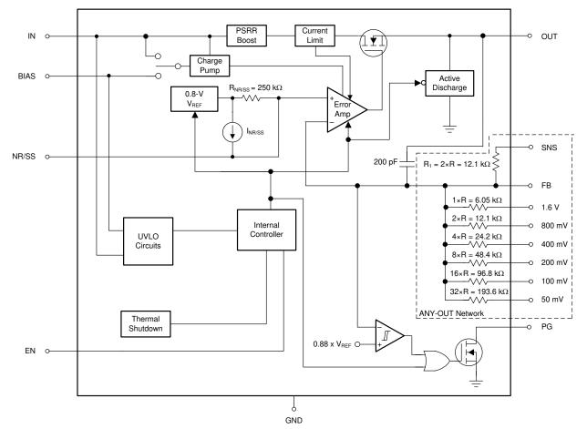
For the ANY-OUT network, the ratios between the values are highly accurate as a result of matching, but the actual resistance may vary significantly from the numbers listed.
