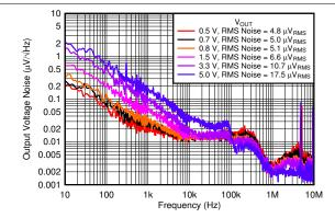
$V_{IN}$  =  $V_{OUT}$  + 0.3 V or  $V_{IN}$  = 1.1 V (whichever is greater),  $V_{BIAS}$  = 5 V for  $V_{IN}$  ≤ 2.2 V,  $I_{OUT}$  = 3 A,  $C_{OUT}$  = 47 μF || 10 μF || 10 μF,  $C_{NR/SS}$  = 10 nF,  $C_{FF}$  = 10 nF, RMS noise BW = 10 Hz to 100 kHz
