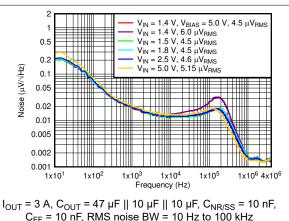
Figure 6-11. Output Noise vs Frequency and VIN
