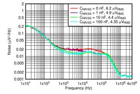
$V_{IN} = V_{OUT} + 0.3 \text{ V, } V_{BIAS} = 5 \text{ V, } I_{OUT} = 3 \text{ A, } C_{OUT} = 47 \text{ }\mu\text{F } ||$  10 \text{ }\text{\$\mu\text{F}\$} || 10 \text{ }\text{\$\mu\text{F}\$} || 10 \text{\$\mu\text{F}\$} || 10 \text{\$\$\mu\text{F}\$} ||
