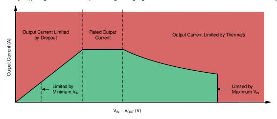
Figure 8-14. Continuous Operation Slope Region Description
