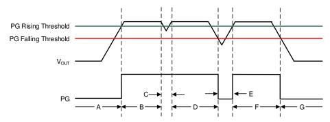
Figure 8-5. Typical PG Operation
