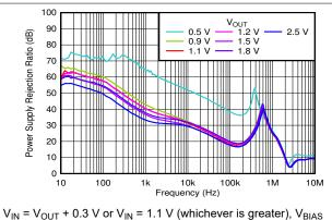
$C_{NR/SS} = 10 \text{ nF}, C_{FF} = 10 \text{ nF}$ Figure 6-47. PSRR vs Frequency and V<sub>OUT</sub> With Bias
