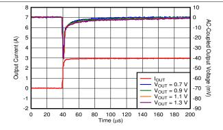
$$\begin{split} V_{\text{IN}} &= V_{\text{OUT}} + 0.5 \text{ V}, V_{\text{BIAS}} = 5 \text{ V}, I_{\text{OUT}} = 100 \text{ mA to 3 A}, \\ \text{slew rate} &= 1 \text{ A/}\mu\text{s}, C_{\text{NR/SS}} = C_{\text{FF}} = 10 \text{ nF}, \\ C_{\text{OUT}} &= 47 \text{ }\mu\text{F} \text{ }|| \text{ }10 \text{ }\mu\text{F} \text{ }|| \text{ }10 \text{ }\mu\text{F} \end{split}$$
