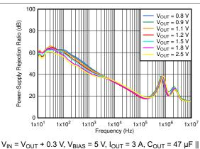
Figure 6-5. PSRR vs Frequency and V<sub>OUT</sub> With Bias
