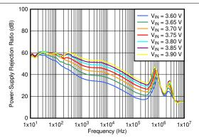
$I_{OUT}$  = 3 A,  $C_{OUT}$  = 47  $\mu F$  || 10  $\mu F$  || 10  $\mu F$  ,  $C_{NR/SS}$  = 10 nF,  $C_{FF}$  = 10 nF
