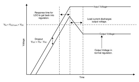
Figure 8-12. Start-Up Into Dropout
