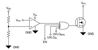
Figure 7-6. Simplified PG Circuit
