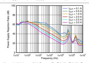
$V_{IN}$  = 1.1 V,  $V_{BIAS}$  = 5 V,  $C_{OUT}$  = 47  $\mu F$  || 10  $\mu F$  || 10  $\mu F$  ,  $C_{NR/SS}$  = 10 nF,  $C_{FF}$  = 10 nF
