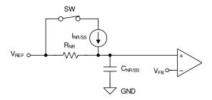
Figure 7-4. Simplified Soft-Start Circuit
