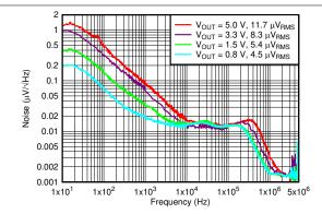
$V_{IN}$  =  $V_{OUT}$  + 0.3 V and  $V_{BIAS}$  = 5 V for  $V_{OUT}$  ≤ 2.2 V,  $I_{OUT}$  = 3 A,  $C_{OUT}$  = 47  $\mu$ F || 10  $\mu$ F || 10  $\mu$ F,  $C_{NR/SS}$  = 10 nF,  $C_{FF}$  = 10 nF, RMS noise BW = 10 Hz to 100 kHz
