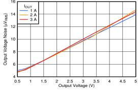
$V_{IN}$  =  $V_{OUT}$  + 0.3 V or  $V_{IN}$  = 1.1 V (whichever is greater),  $V_{BIAS}$  = 5 V for  $V_{IN}$  ≤ 2.2 V,  $C_{OUT}$  = 47  $\mu$ F || 10  $\mu$ F || 10  $\mu$ F,  $C_{NR/SS}$  = 10 nF,  $C_{FF}$  = 10 nF, RMS noise BW = 10 Hz to 100 kHz
