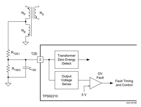
Figure 26. TZE and Output Overvoltage Detection
