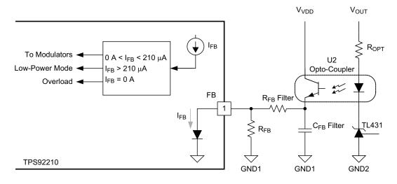
Figure 23. FB Pin Details for Peak-Current Mode Control
