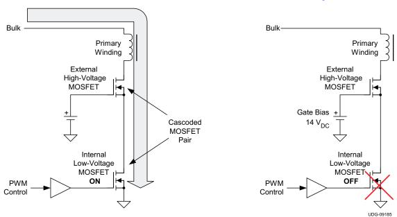
Figure 18. Cascoded Architecture
