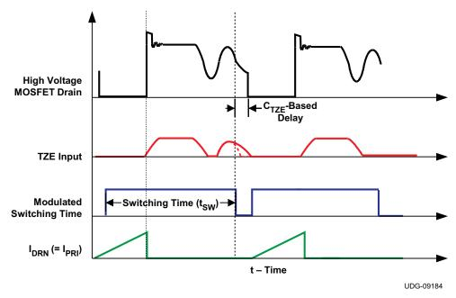
Figure 25. TZE and HVMOSFET Drain Voltages for Valley Switching
