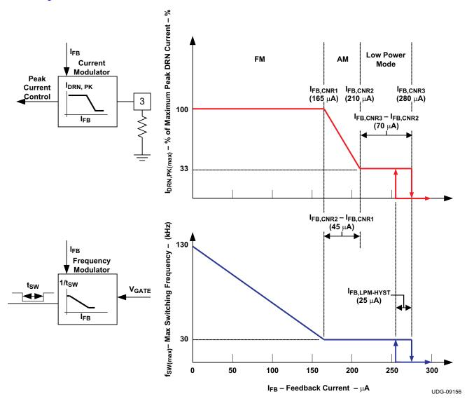
Figure 24. FB Pin Based Modulation Modes
