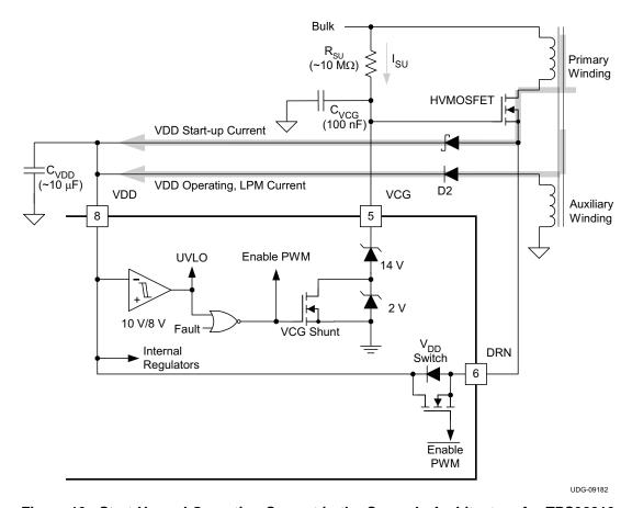
Figure 19. Start-Up and Operating Current in the Cascode Architecture for TPS92210
