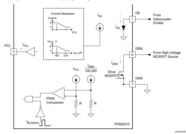
Figure 20. Peak Current Limit (PCL) Pin Details
