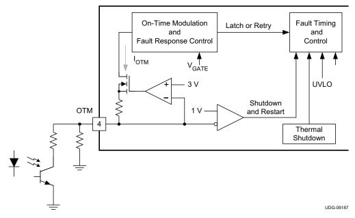
Figure 21. On-Time Modulation Detail
