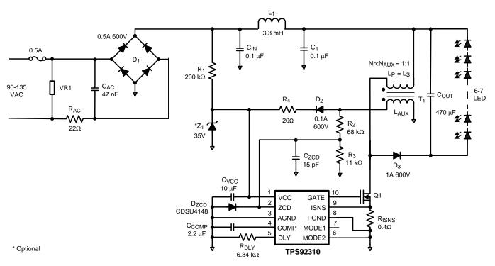
Figure 26. Non-isolated topology schematic
