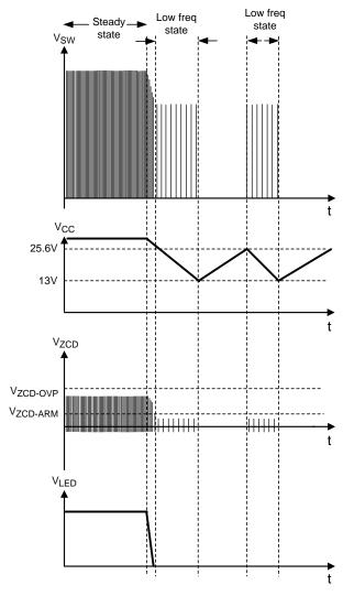
Figure 19. Output Short Circuit waveforms
