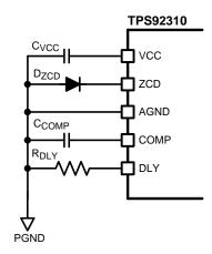
Figure 23. Compensation and DLY Timer connection
