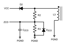
Figure 22. Auxiliary Winding Interface to ZCD
