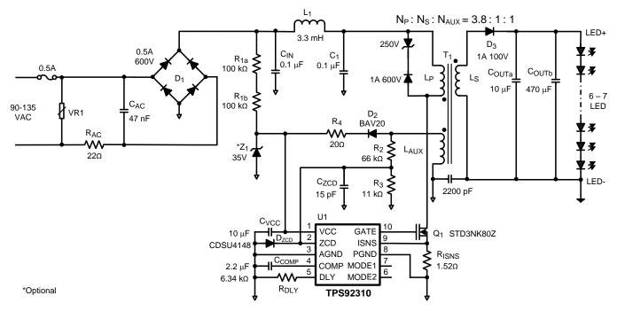
Figure 25. Isolated topology schematic
