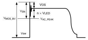
Figure 24. Snubber Waveform
