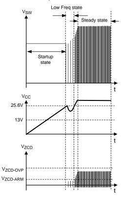
Figure 16. Start up Bias Waveforms
