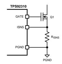
Figure 21. R<sub>ISNS</sub> Resistor Interface
