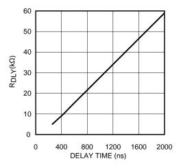
Figure 18. Delay Time Setting
