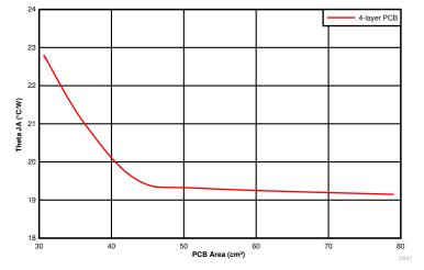
Figure 10-4. R<sub>0JA</sub> versus PCB Area (per Layer)
