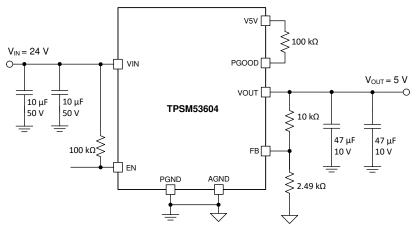
Figure 8-1. TPSM53604 Typical Schematic
