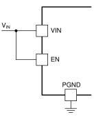
Figure 7-3. Enabling the Device
