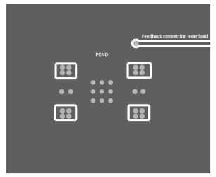
Figure 10-3. Typical PGND Layer
