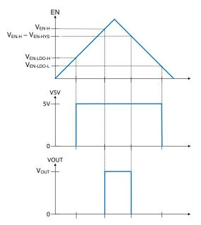
Figure 7-2. Precision Enable Behavior
