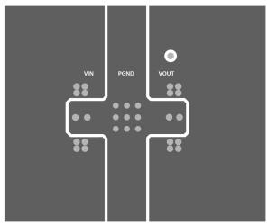
Figure 10-1. Typical Top-Layer Layout
