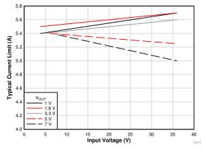
Figure 7-13. Current Limit Threshold
