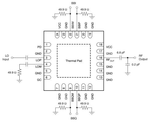
(1) Pin 1 (PD) and Pin 6 (GC) are internally pulled down.
