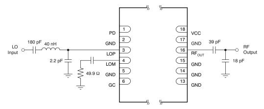
Figure 66. Matching Components for Operation Centered at 350 MHz
