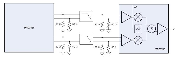
Figure 67. DAC348x Interface with the TRF3705 Modulator
