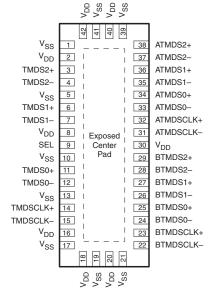
For RUA, the exposed center pad must be connected to  $V_{SS}$  or electronically open. For this part to be used in HDMI/TMDS applications,  $V_{SS}$  can be elevated to 1.5 V. See Figure 1.
