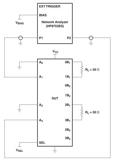
Figure 7. Test Circuit for Crosstalk (X<sub>TALK</sub>)
