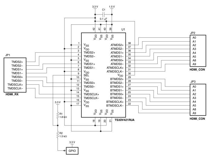
Figure 9. Reference Circuit for HDMI Application
