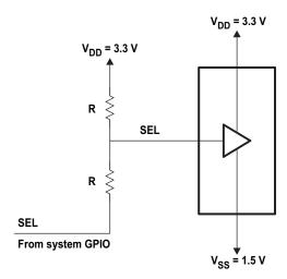
This example circuit shows connecting control inputs to GPIOs of an application using  $V_{SS} = 1.5 \text{ V}$ , which allows the device to pass TMDS signal levels
