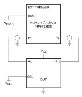
Figure 6. Test Circuit for Frequency Response (BW)
