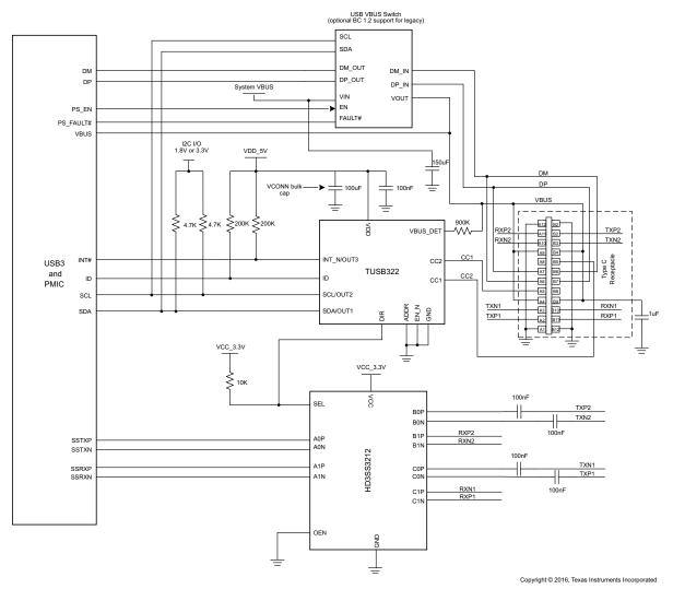
Figure 10. DFP in I<sup>2</sup>C Mode Schematic
