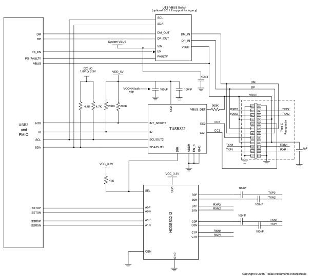
Figure 8. DRP in I<sup>2</sup>C Mode Schematic
