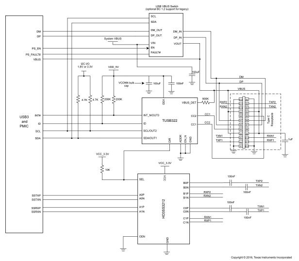
Figure 12. UFP in I<sup>2</sup>C Mode Schematic
