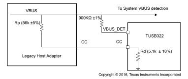
Figure 2. Legacy Adapter Implementation Circuit
