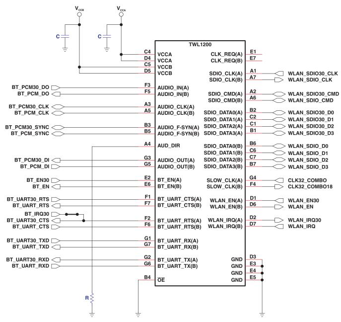
Figure 25. Application Circuit Example, OE Connection With Audio\_CLK and Audio\_F-SYNC Channels Established From B Side to A Side
