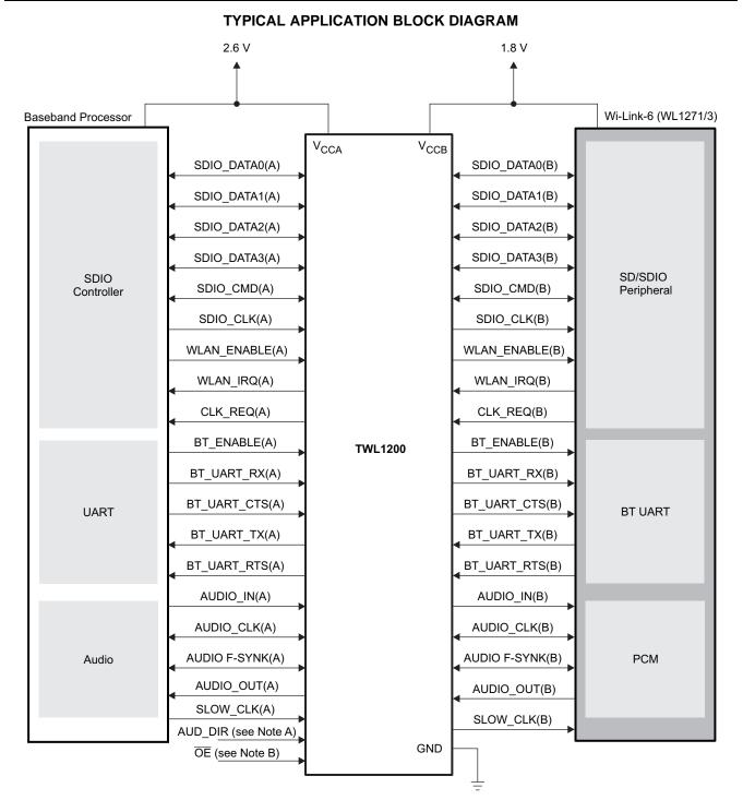
A. AUD\_DIR must be biased to determine audio direction (see Function Table for properly establishing the bias).
