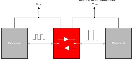
Typical Application Block Diagram for TXB010X
