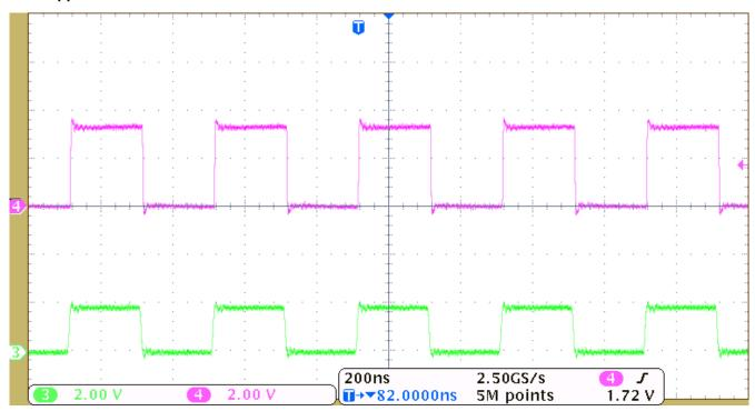
Figure 9-2. Example of Level Translation of a 2.5-MHz 1.8 V Signal (Green) to a 3.3 V Signal (Pink)
