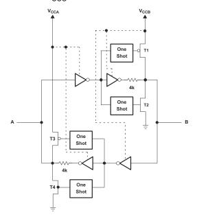
Figure 8-1. Architecture of TXB0104 I/O Cell
