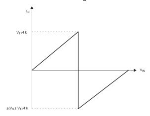
Figure 8-2. Typical I<sub>IN</sub> vs V<sub>IN</sub> Curve
