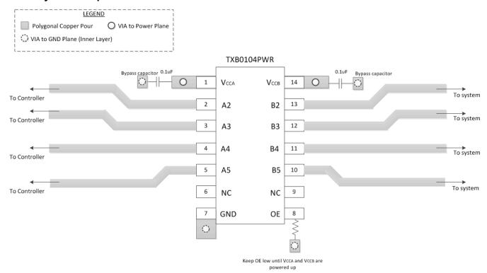
Figure 11-1. Layout Example Schematic
