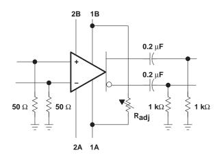
**VOLTAGE AMPLIFICATION ADJUSTMENT**
