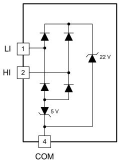
Figure 31. Diode Structure of Input Stage
