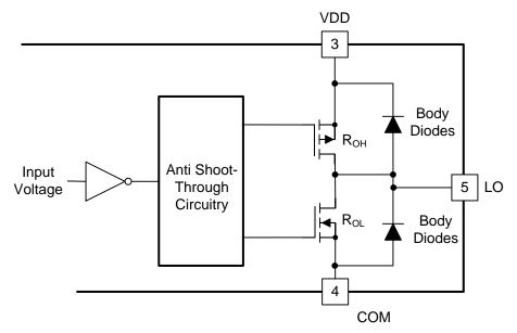
Figure 32. Output Stage Structure
