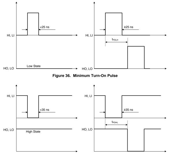
Figure 37. Minimum Turn-Off Pulse
