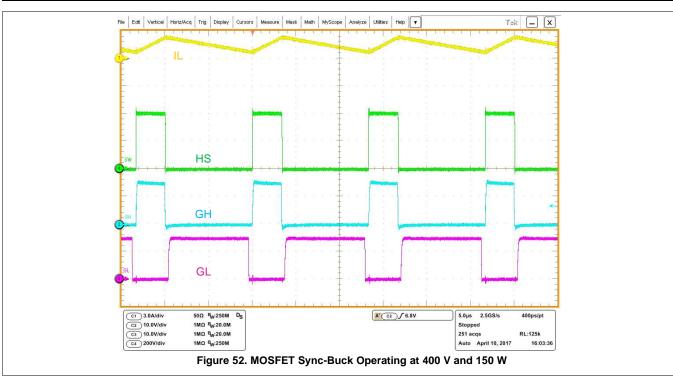
Figure 52 shows UCC27712-Q1 operating in a high voltage sync-buck. Channel 1 depicts inductor current, Channel 2 high side MOSFET VGS, Channel 3 low side MOSFET VGS, and Channel 4 high voltage switch node.
