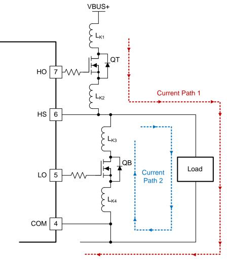
Figure 40. HS Negative Voltage In Half-Bridge Configuration
