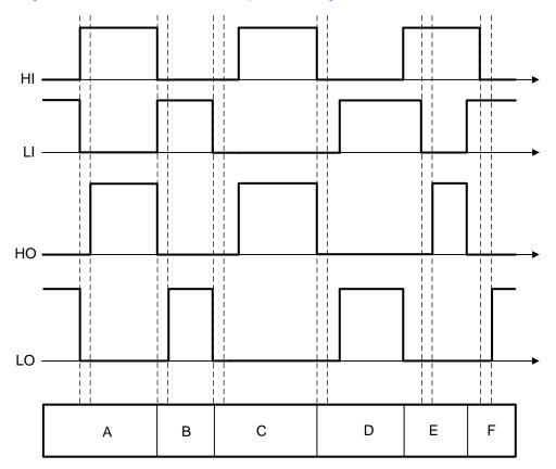
Figure 39. Input and Output Logic Relationship
