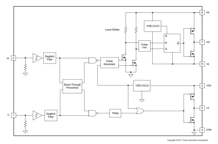
Figure 29. UCC27712-Q1 Block Diagram
