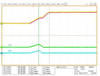
Figure 45. VDD/HB-HS Fast Ramp Up
