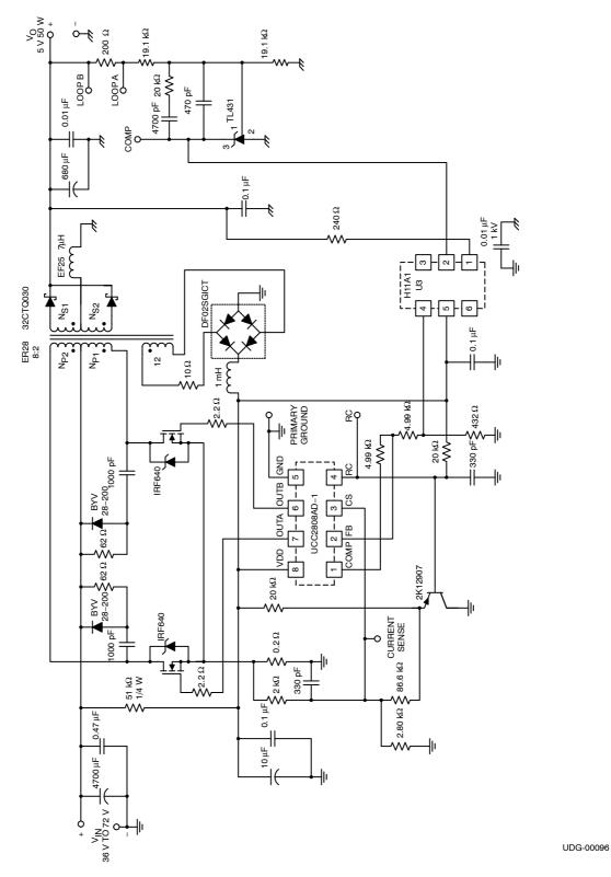
Figure 2. Typical Application Diagram: 48-V In, 5-V, 50-W Output
