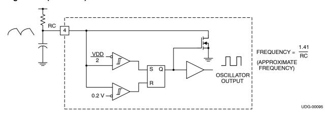
Figure 1. Block Diagram for Oscillator
