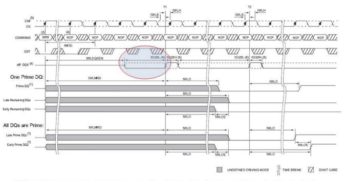
NOTES: 1. DRAM has the option to drive leveling feedback on a prime DQ or all DQs. If feedback is driven only on one DQ, the remaining DQs must be driven low, as shown in above Figure, and maintained at this state through out the leveling procedure.
