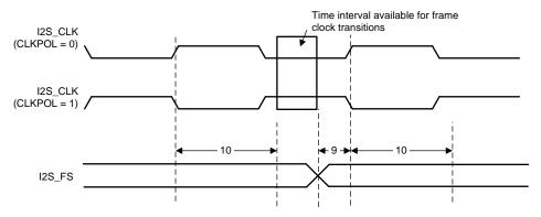
Figure 5. I2S Frame Clock Timing Constant
