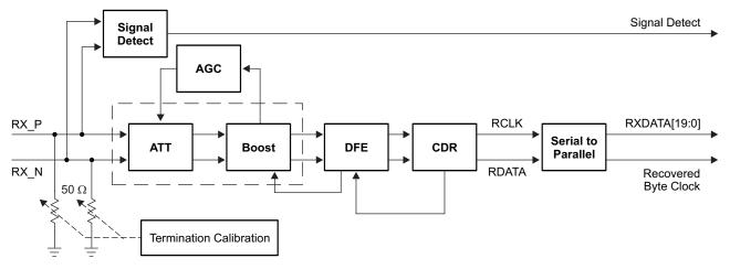
Figure 10. RX Path Block Diagram
