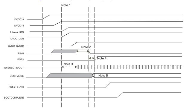
Figure 3 shows the power sequencing diagram when HF OSC.
