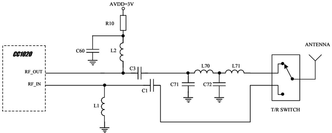
**Figure 1: Schematic diagram of the input/output matching network**
