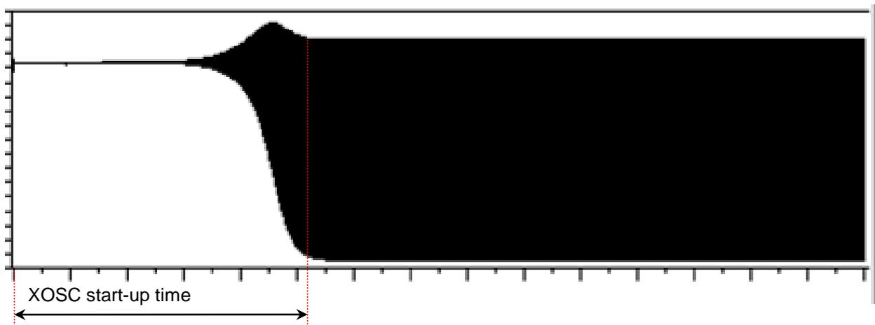
When finding the max start-up time one should measure on several crystals over temperature. A 100% margin should be added to the measured start-up time to account for process variations.
