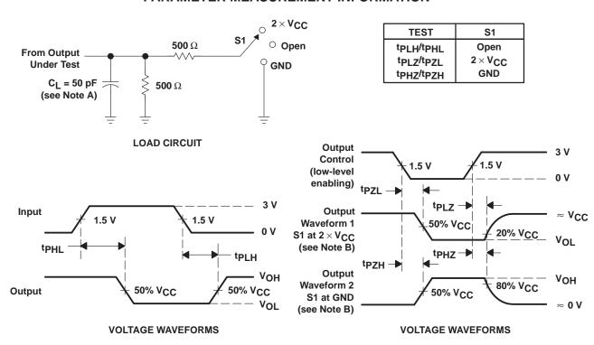
NOTES: A. C<sub>L</sub> includes probe and jig capacitance.
