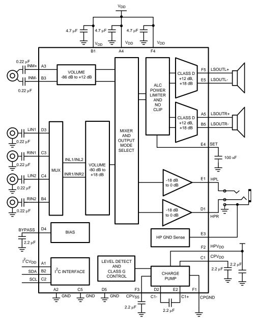
Figure 2. Typical Audio Amplifier Application Circuit
