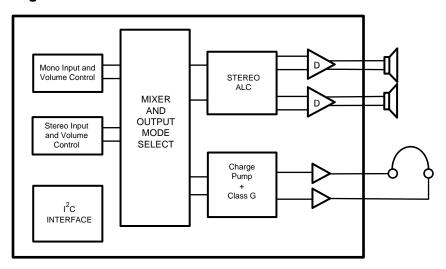
Figure 1. LM49251 Simplified Block Diagram
