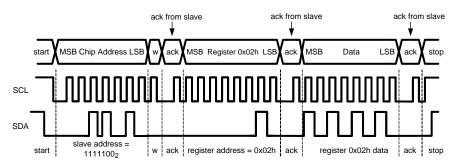
Figure 51. Example I<sup>2</sup>C Write Cycle
