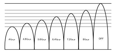
Figure 55. Voltage Limit Output Level
