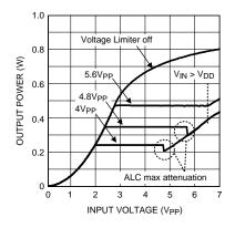
Figure 58. Voltage Limiter Function  $V_{DD} = 3.3V$ ,  $R_L = 15\mu H + 8\Omega + 15\mu H$   $f_{IN} = 1kHz$ ,  $LS\_GAIN = 0$
