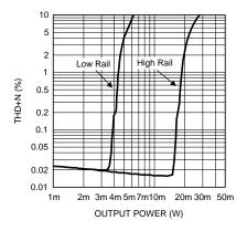
Figure 54. Class G Disabled (Low/High Supply Rails)
