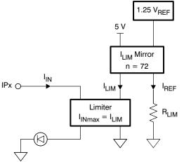
Figure 13. Digital Input Stage
