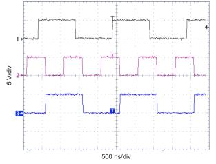
Figure 25. SN65HVS883 Serial Input and Output Timing
