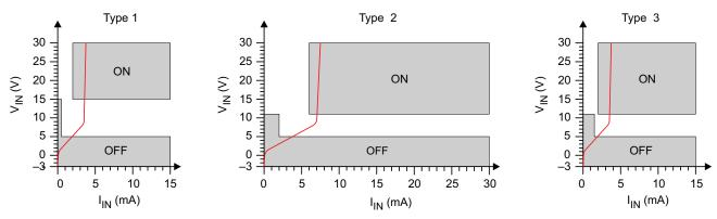
Figure 18. Switching Characteristics for IEC61131-2 Type 1, 2, and 3 Proximity Switches
