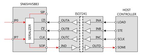
Figure 20. Simple Isolation of the Shift Register Interface
