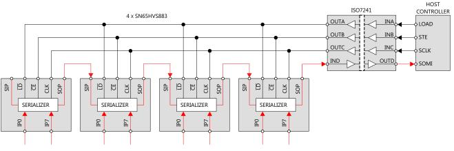
Figure 22. Cascading Four SN65HVS883 for a 32-Channel Input Module
