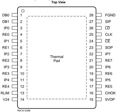
PWP Package 28 Pin (HTSSOP) With Exposed Thermal Pad Top View
