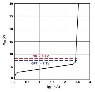
Figure 24. SN65HVS883 Example Input Characteristic
