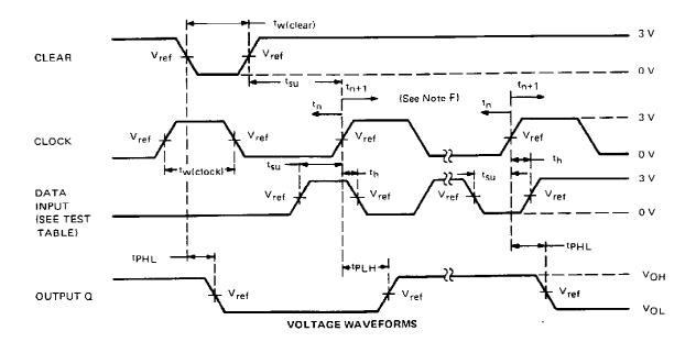
NOTES: A. The clock pulse generator has the following characteristics:  $Z_{out}\approx 50~\Omega$  and PRR  $\leqslant$  1 MHz, For '194,  $t_r\leqslant$  7 ns and  $t_f\leqslant$  7 ns. For 'LS194A,  $t_r\leqslant$  15 ns and  $t_f\leqslant$  6 ns. For 'S194,  $t_r\leqslant$  2.5 ns and  $t_f\leqslant$  2.5 ns. When testing  $f_{max}$ , vary PRR.
