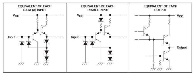
Figure 7-1. Schematics of Inputs and Outputs
