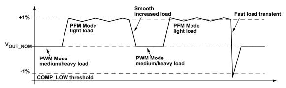
Figure 7. Dynamic Voltage Positioning
