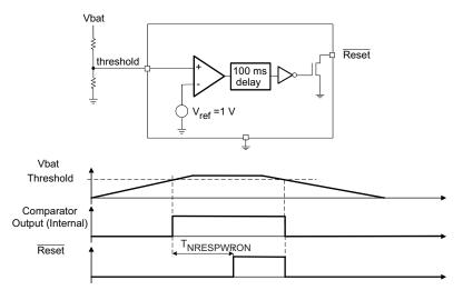
Figure 6. RESET Pulse Circuit
