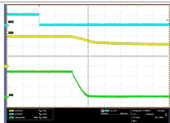
Ch. 1 =  $V_{(OUT)}$       Ch. 2 =  $V_{(PWM)}$       Ch. 4 =  $I_{(OUT)}$
