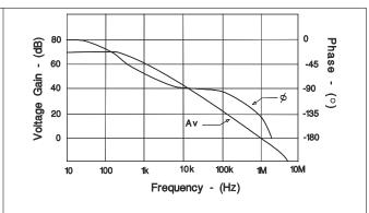
Figure 6-2. Error Amplifier Open-Loop Frequency Response
