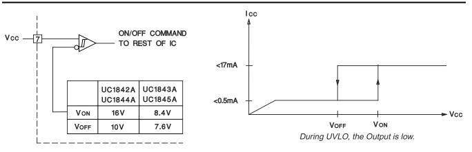
Figure 7-3. Undervoltage Lockout
