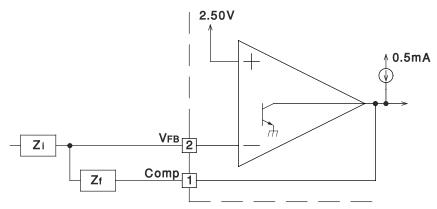
Figure 7-2. Error Amplifier Configuration Diagram
