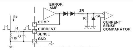
Figure 7-1. Current Sense Circuit Diagram
