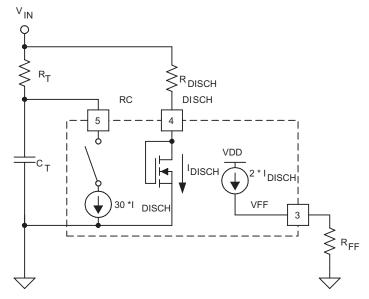
Figure 3. Duty Cycle Clamp (MODE = 1)
