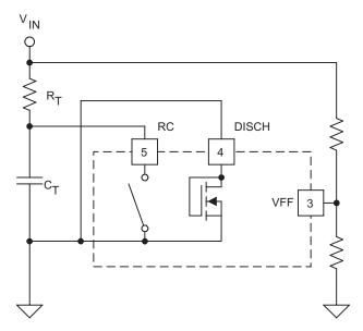
Figure 4. Ocsillator Without Clamp (MODE = 0)
