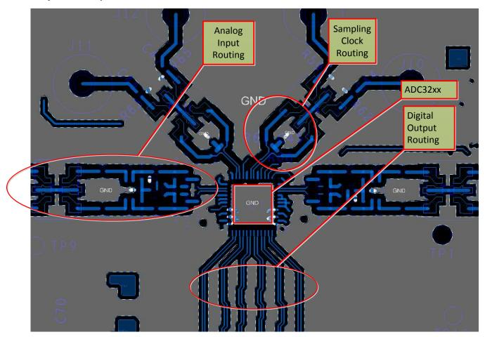
Figure 91. Typical Layout of the ADC3244E Board
