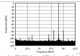
$$\begin{split} f_{\text{IN}} = 170.1 & \text{MHz, } f_{\text{CMRR}} = 5 & \text{MHz, } A_{\text{CMRR}} = 50 & \text{mV}_{\text{PP}}, \\ \text{SNR} = 69.72 & \text{dBFS, SINAD} = 69.66 & \text{dBFS, SFDR} = 75.66 & \text{dBc,} \\ \text{THD} = -86.98 & \text{dBc, SFDR} = 75.66 & \text{dBc (non 23)} \end{split}$$
