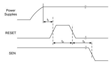
Figure 57. Initialization of Serial Registers after Power-Up
