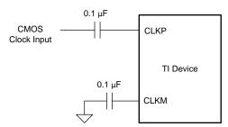
Figure 47. Single-Ended Clock Driving Circuit
