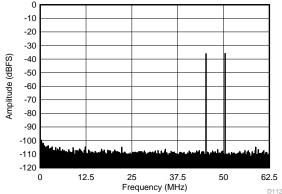
$f_{\text{IN1}}$  = 46 MHz,  $f_{\text{IN2}}$  = 50 MHz, IMD3 = 90.8 dBFS, each tone at –36 dBFS
