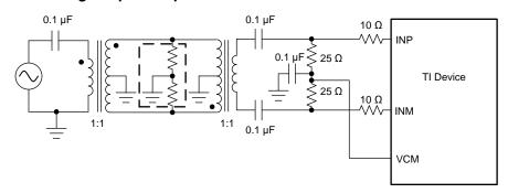
Figure 89. Driving Circuit for High input Frequencies (f<sub>IN</sub> > 230 MHz)
