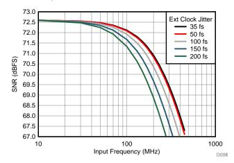
Figure 48. SNR vs Frequency for Different Clock Jitter
