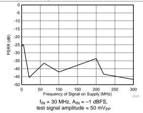
Figure 32. Power-Supply Rejection Ratio vs Test Signal Frequency
