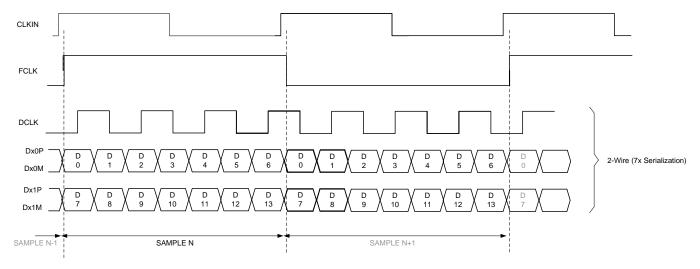
Figure 49. Output Timing Diagram
