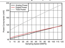
Figure 36. Power vs Sampling Frequency (1-Wire Mode)
