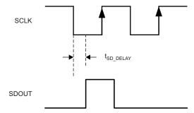
Figure 56. SDOUT Timing Diagram
