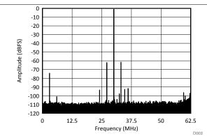
$$\begin{split} f_{IN} = 30.1 & \text{MHz, } f_{PSRR} = 3 & \text{MHz, } A_{PSRR} = 50 & \text{mV}_{PP}, \\ \text{SNR} = 58.51 & \text{dBFS, } \text{SINAD} = 58.51 & \text{dBFS, } \text{SFDR} = 60.53 & \text{dBc,} \\ \text{THD} = -90.71 & \text{dBc, } \text{SFDR} = 60.53 & \text{dBc (non 23)} \end{split}$$
