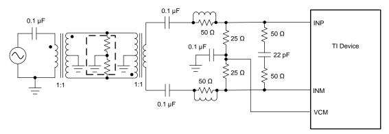
Figure 85. Driving Circuit for Low Input Frequencies
