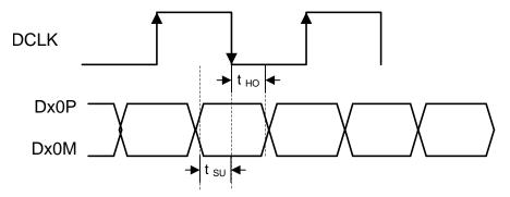
Figure 41. Setup and Hold Time
