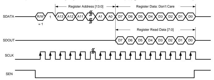
Figure 55. Serial Register Read Timing Diagram
