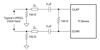
Figure 45. LVPECL Clock Driving Circuit
