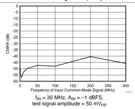
Figure 34. Common-Mode Rejection Ratio vs Test Signal Frequency
