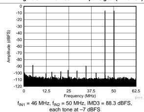
Figure 11. FFT for Two-Tone Input Signal
