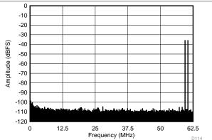
$f_{\text{IN1}}$  = 185 MHz,  $f_{\text{IN2}}$  = 190 MHz, IMD3 = 87.28 dBFS, each tone at -36 dBFS
