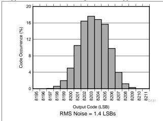
Figure 31. Idle Channel Histogram
