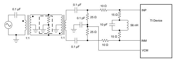
Figure 87. Driving Circuit for Mid-Range Input Frequencies (100 MHz < fin < 230 MHz)
