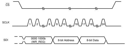
Figure 7-9. Register Write Operation
