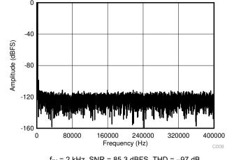
Figure 8-2 shows the FFT plot for the ADS7067 with a 2-kHz input frequency used for the circuit in Figure 8-1.
