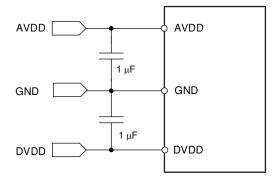
Figure 9-1. Power-Supply Decoupling
