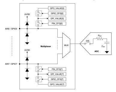
Figure 7-1. Analog Inputs, GPIOs, and ADC Connections
