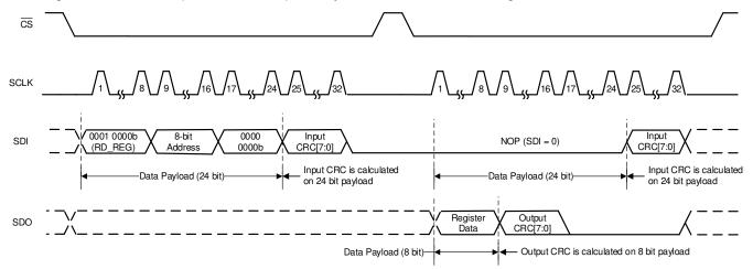
Figure 7-11. Register Read With CRC
