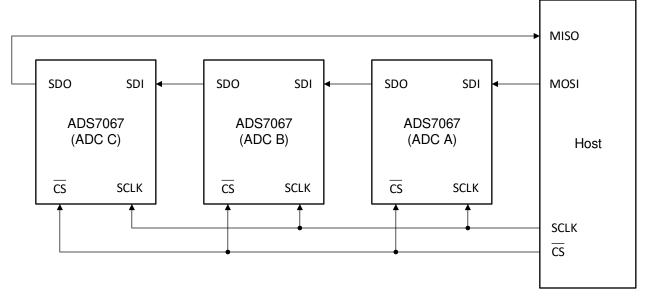
Figure 7-7. Multiple Converters Connected Using Daisy-Chain Mode
