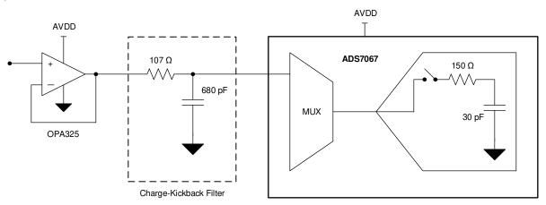
Figure 8-1. DAQ Circuit: Single-Supply DAQ
