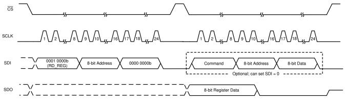
Figure 7-10. Register Read Operation
