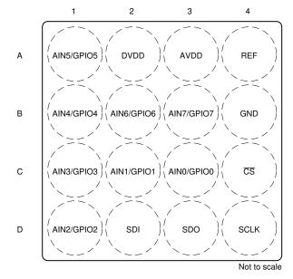
Figure 5-1. YBH Package, 16-Pin WCSP, Top View
