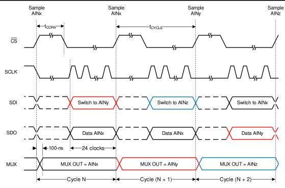
Figure 7-13. Starting a Conversion and Reading Data in Manual Mode
