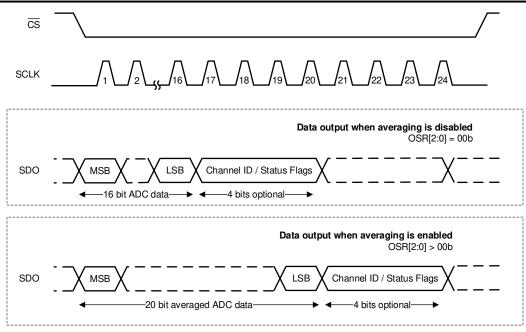
Figure 7-4. SPI Frames for Reading Data
