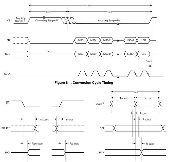
Figure 6-2. SPI Interface Timing
