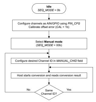
Figure 7-12. Device Operation in Manual Mode
