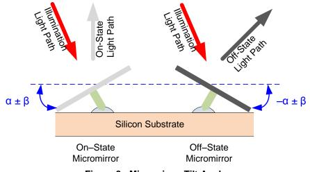
Figure 8. Micromirror Tilt Angle
