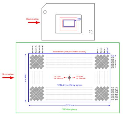
Figure 6. Micromirror Array Physical Characteristics
