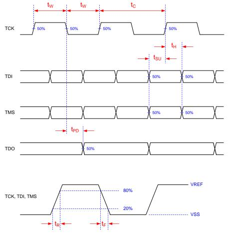
Figure 3. JTAG Boundary Scan Control Logic Timing Requirements
