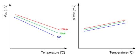
Figure 11. Example of Delta VBE vs Temperature
