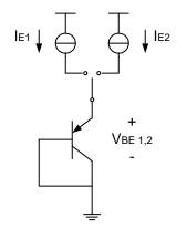
Figure 10. Temperature Measurement Theory
