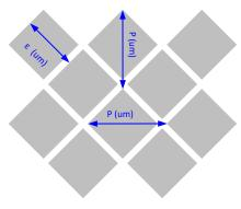
Figure 7. Mirror (Pixel) Pitch
