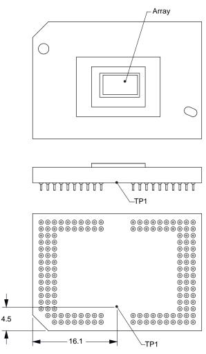
Figure 12. Thermocouple Locations
