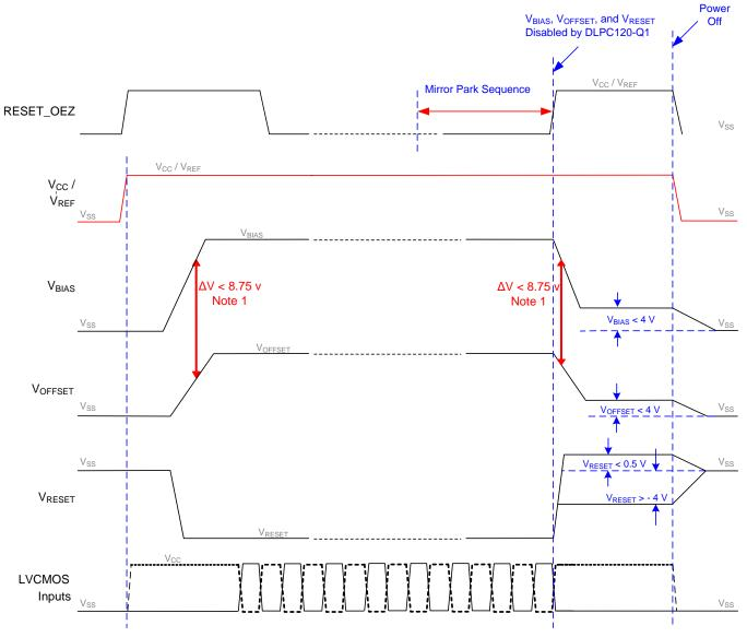
(1) ±8.75-V delta,  $\Delta V$ , shall be considered the max operating delta between V<sub>BIAS</sub> and V<sub>OFFSET</sub>. Customers may find that the most reliable way to ensure this is to power V<sub>OFFSET</sub> prior to V<sub>BIAS</sub> during power up and to remove V<sub>BIAS</sub> prior to V<sub>OFFSET</sub> during power down.
