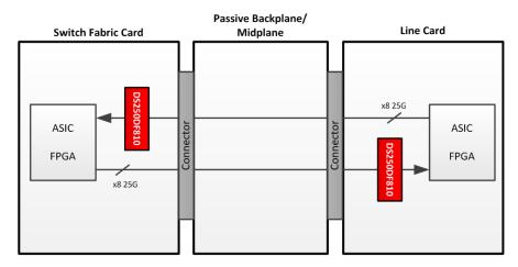
Figure 16. Backplane/Mid-plane Application Block Diagram
