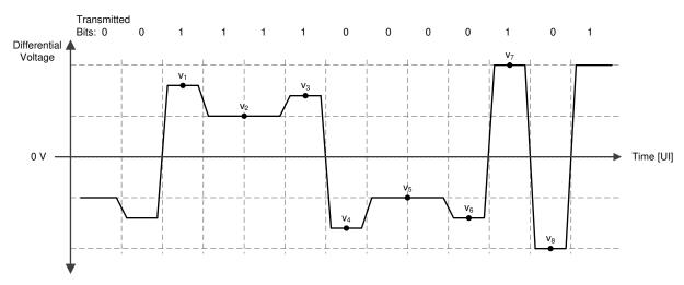
Figure 8. Conceptual FIR Waveform With Post-Cursor Only
