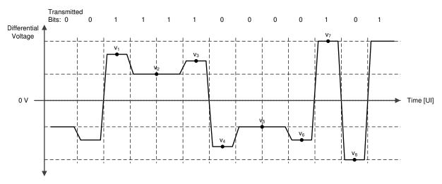
Figure 10. Conceptual FIR Waveform With Both Pre- And Post-Cursor
