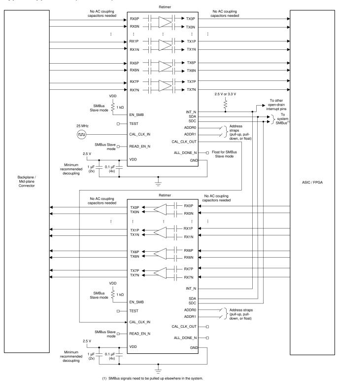
Figure 17. Backplane/Mid-plane Application Schematic
