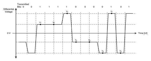
Figure 9. Conceptual FIR Waveform With Pre-Cursor Only
