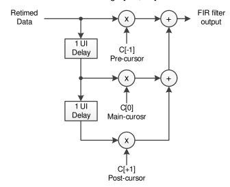
Figure 7. FIR Filter Functional Model
