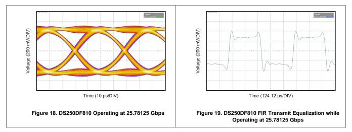
Figure 18 shows a typical output eye diagram for the DS250DF810 operating at 25.78125 Gbps with PRBS9 pattern using FIR main-cursor of +18, pre-cursor of -1 and post-cursor of +2. All other device settings are left at default.
