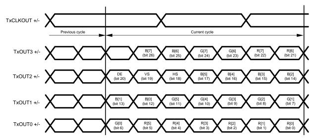
Figure 16. 8-bit FPD-LInk Mapping: MSB's on TxOUT3
