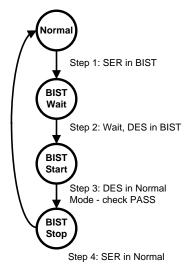
Figure 19. BIST Mode Flow Diagram
