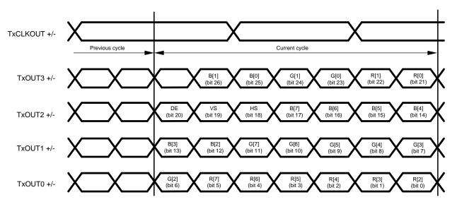
Figure 15. 8-bit FPD-LInk Mapping: LSB's on TxOUT3
