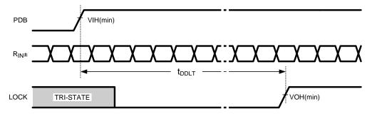
Figure 7. PLL Lock Times
