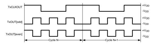
Figure 2. Checkerboard Data Pattern
