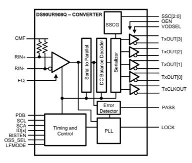
Figure 1. FPD-Link II to FPD-Link Convertor
