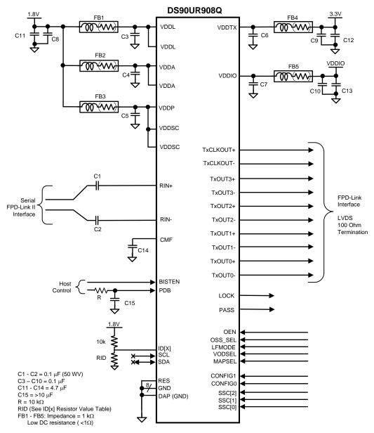
Figure 25. DS90UR908Q Typical Connection Diagram
