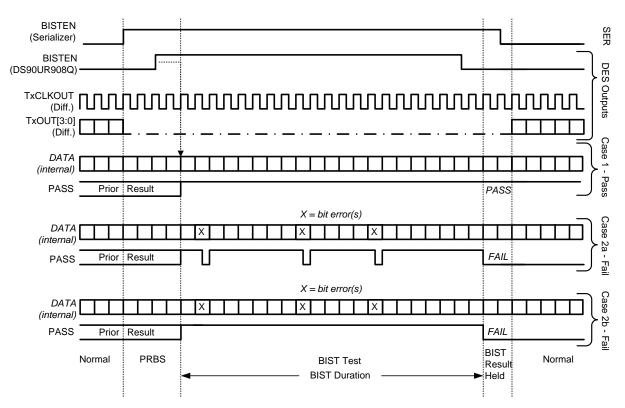
Figure 20. BIST Waveforms
