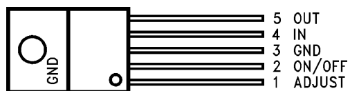
Figure 8. TO-220 5-Lead Power Package Front View
